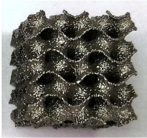
Figure 15. A TPMSS specimen with 0.4 mm wall thickness [91]. Copyright© 2021 Evsevlev et al. CC BY 4.0.
